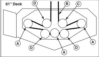
Figure 45. Mower PTO Belt Routing
